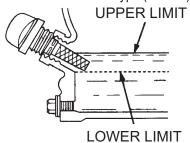
Figure 6. Engine Oil Dipstick
